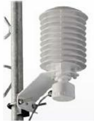
Figure 57 - Temperature measurement instrument (AWS Truepower, 2010)
