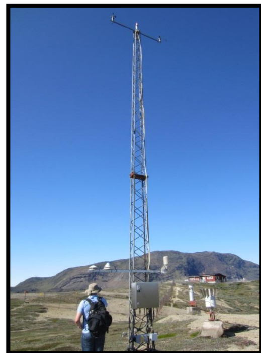
Figure 179 - Met mast in Narsaq with cup anemometer and wind vane
