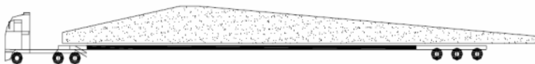
Figure 110 - Semi trailer, rotor blade transportation
