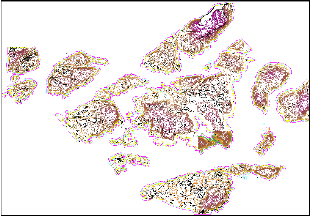
Figure 5: Roughness and orography vector map used in WAsP.
