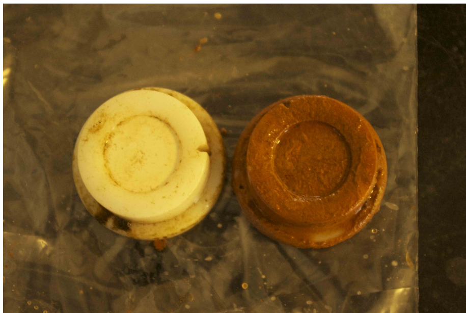
Figure 5.7: Layer of dirt blocking the diffusive layers of the DGT (Å1 on the left, Å3 on the right)
