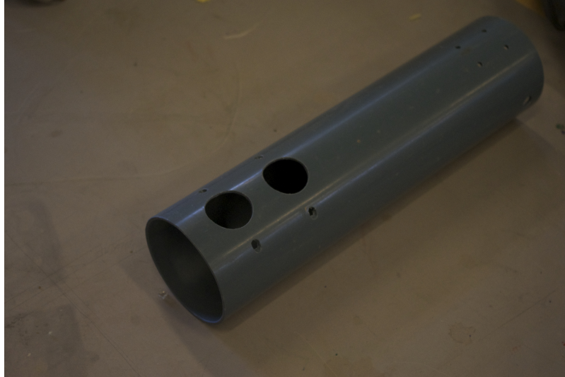
Figure 4.2: Plastic cylinder with holes to place the DGTs
