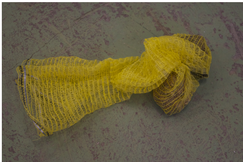
Figure 4.5: Web with stones inside to keep the DGTs below the sea surface
