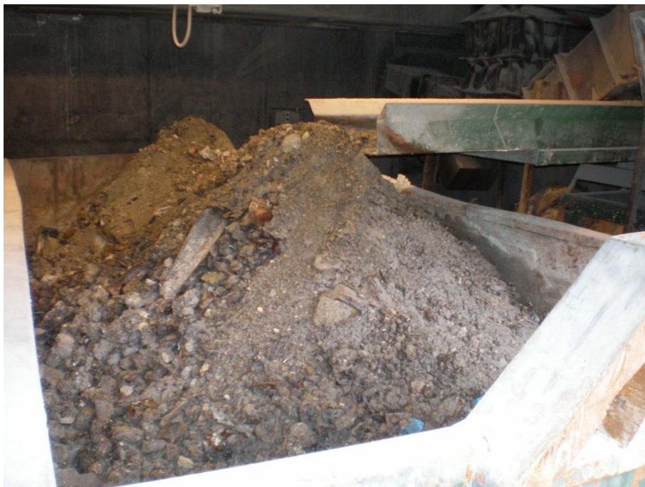
FIGURE 19: BOTTOM ASH CONTAINER, IN THE RESIDUAL AREA OF THE WASTE INCINERATOR.
