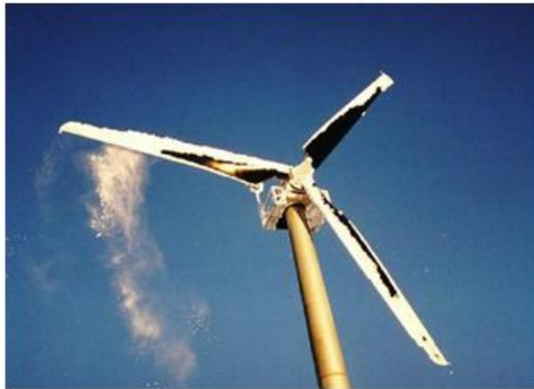
Figure 24: Ice break off with StaClean®.
