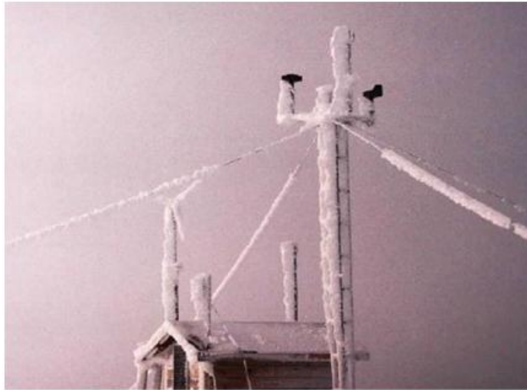
Figure 20: rime ice on met.mast.
