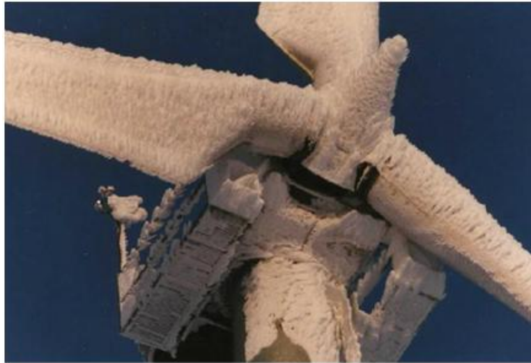
Figure 21: rime ice on the rotor of the 150 kW Mark III turbine.
