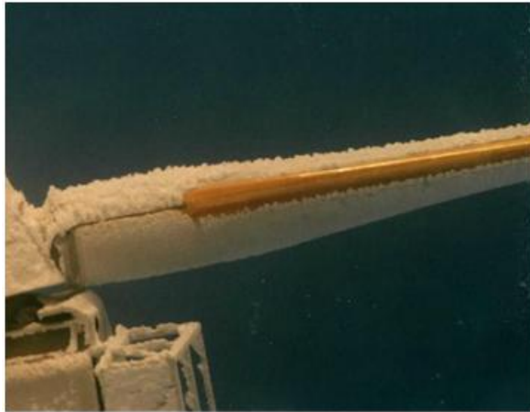
Figure 23: rime ice building up around the blade of the 150 kW Mark III turbine.
