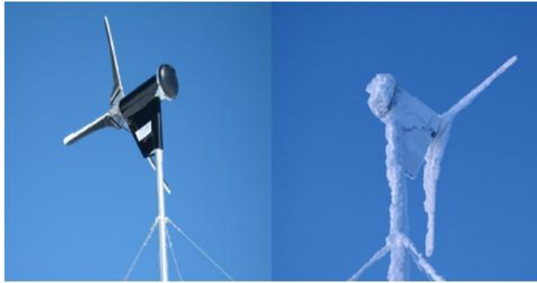
Figure 18: Two different ice build-up levels in the Proven wind turbine.
