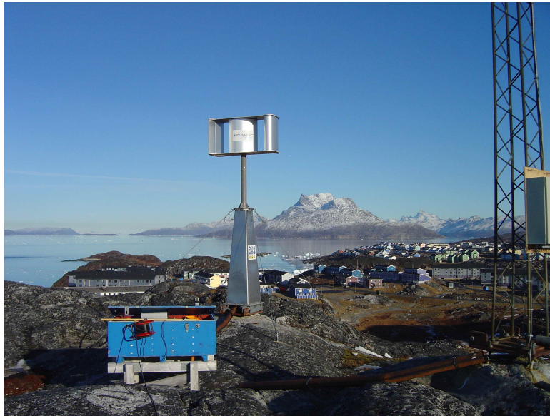
Figure 60: picture of the Ropatec VAWT provided by TELE Greenland A/S.
