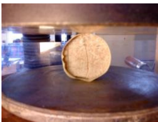
Figure 23: Specimen failure in Brazilian indirect tension.
