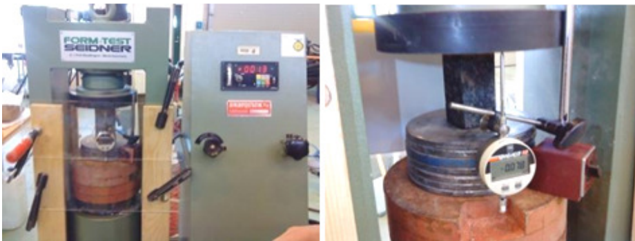
Figure 24: Test setup for unconfined compressive tests.
