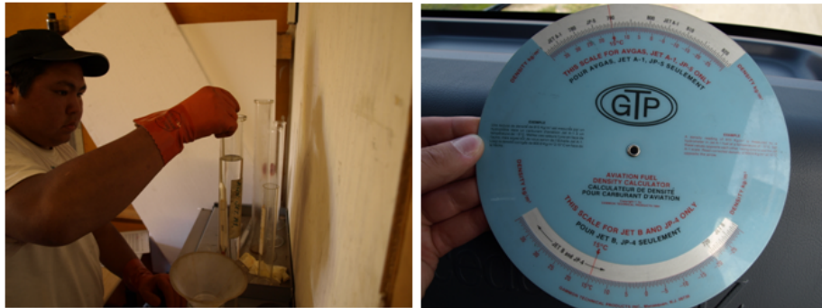
Figure 13: Density measurement of Jet A-1
