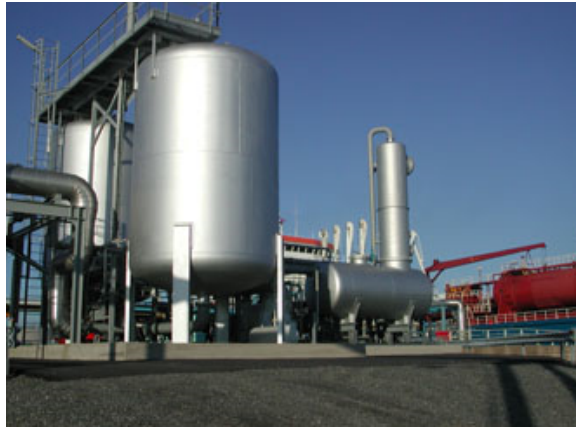
Figure 10: An example of VRU installation [6]
